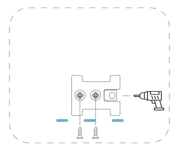
**Caution:** Do not overtighten screws. Screws must be flush with the mounting bracket. Use # 4 Flat Head screws only. The mounting bracket should be level and installed flush to the wall or ceiling surface material.
